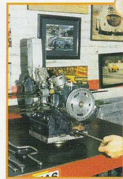
4 Tuercas monoblock 13 mm torqueadas a 14 Ft.-Lbs.
