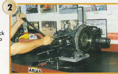
1 Tuercas monoblock 13 mm torqueado a 14 Ft.-Lbs.
